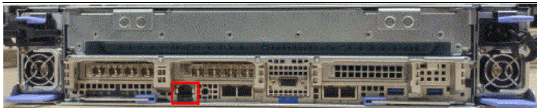
Figure 2-8 Technician port IBM SAN Volume Controller 2145-SV2
