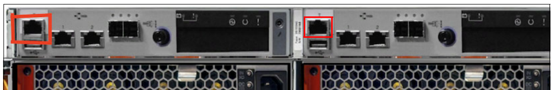
Figure 2-5 Technician port FlashSystem 5045
