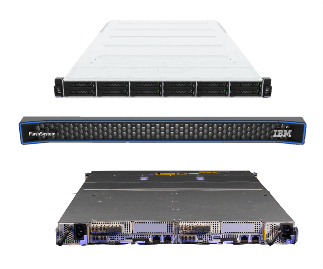
Figure 3 IBM FlashSystem 5300 control enclosure showing the front and rear view
