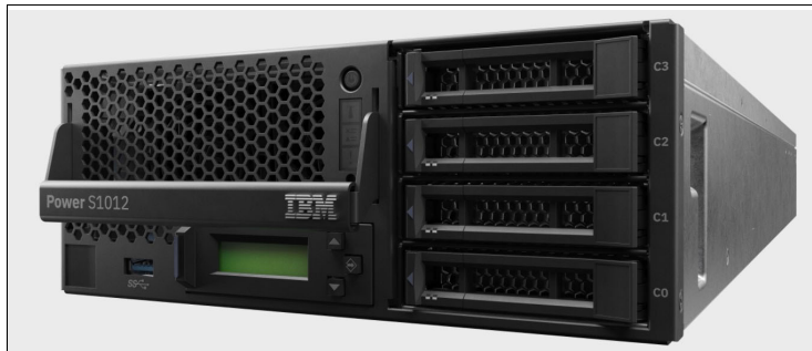
Figure 2-1 Rack mount version of a single Power S1012 System (sled)
