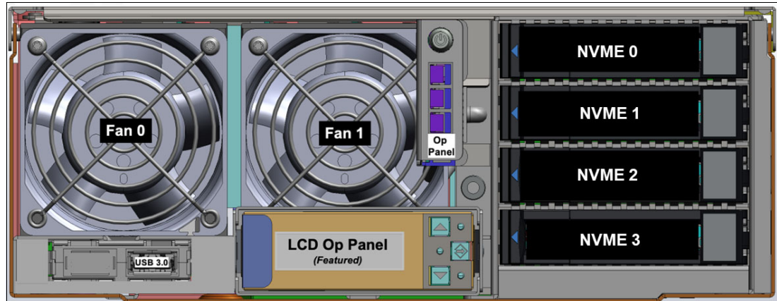
Figure 2-10 NVMe drive placement
