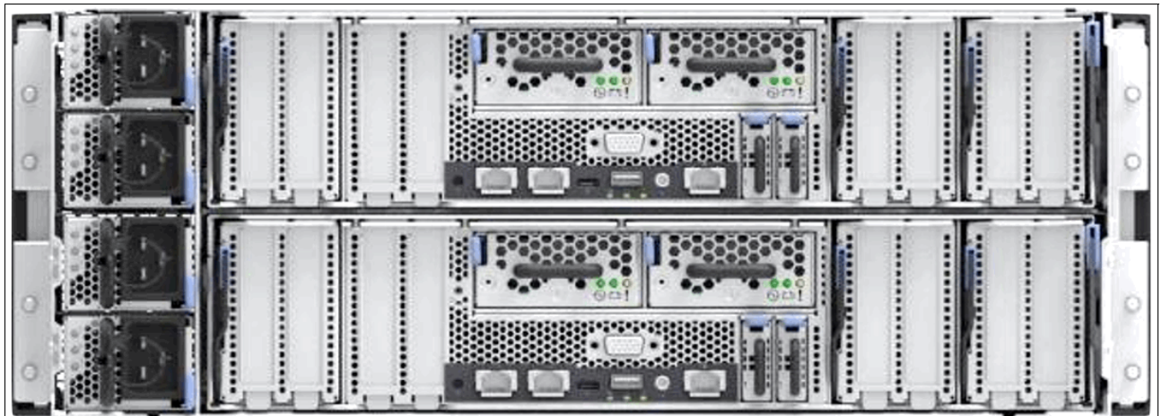
Figure 13 Rear view of IBM FlashSystem 9500 control enclosure
