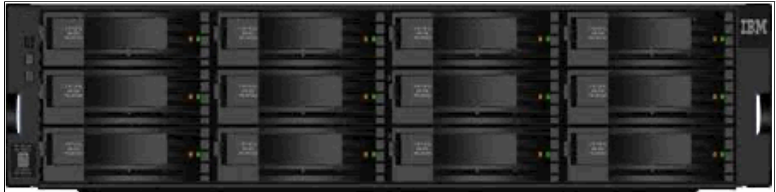
Figure 11 Front view of the IBM FlashSystem 7000 LFF Expansion Enclosure Model 12G
