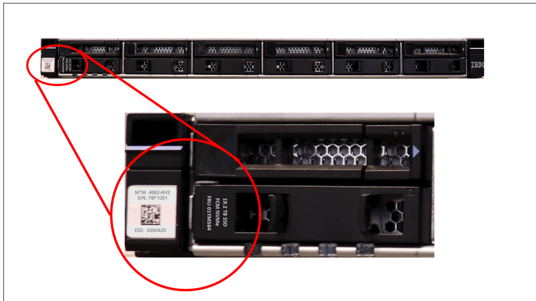
Figure 2 IBM FlashSystem 5200 bezel and IBM FlashCore Module description
