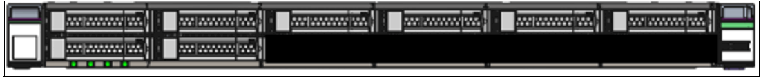
Figure 23 IBM FlashSystem 5200 NVMe drive slots supported by eight drives that are populated and four fillers
