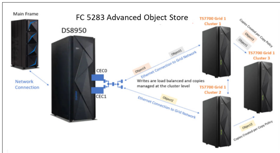
Figure 3-3 DS8000 with advanced object store configured
