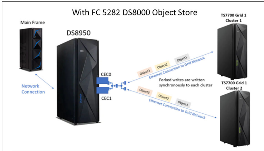
Figure 3-2 DS8000 object store configured
