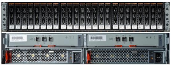
Figure 5 HPFE Gen2 front (top) and rear (bottom)
