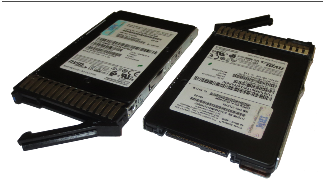
Figure 1-8 Two NVMe devices
