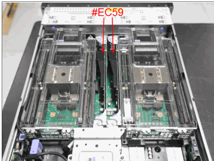
Figure 2-17 Two #EC59 feature codes in a Power S922 server
