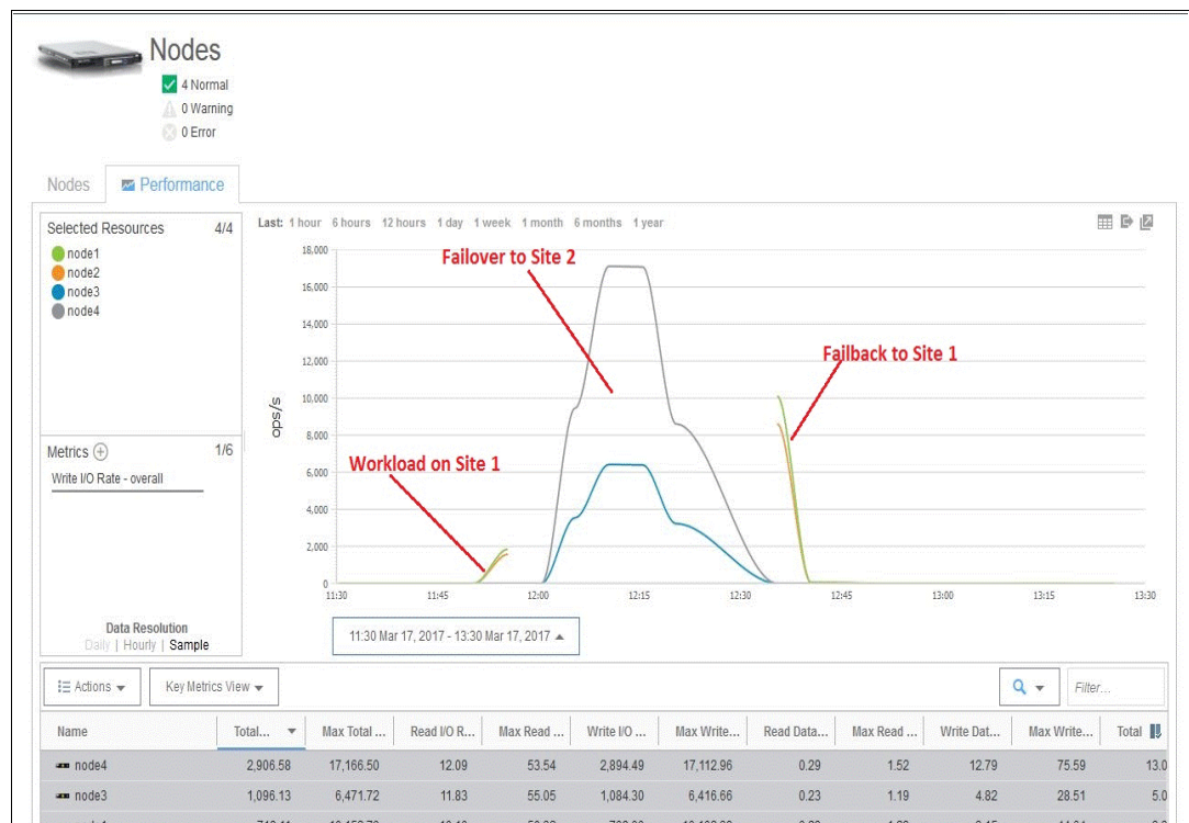
Figure 5-1 Test: I/O group on Site 1 fails
