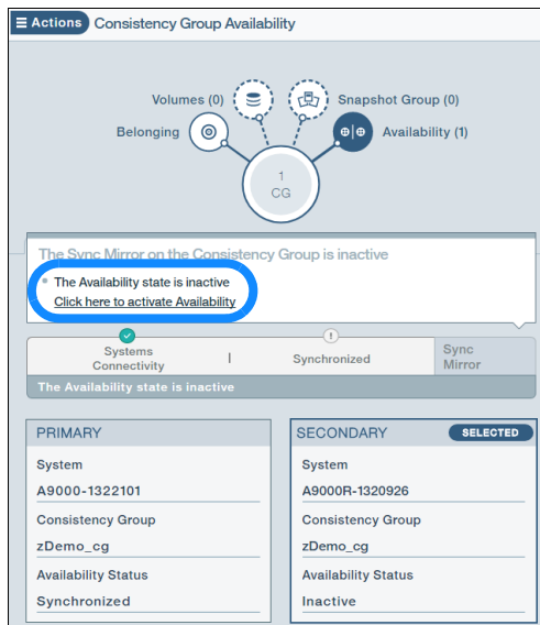
Figure 4-53 Reactivating the consistency group
