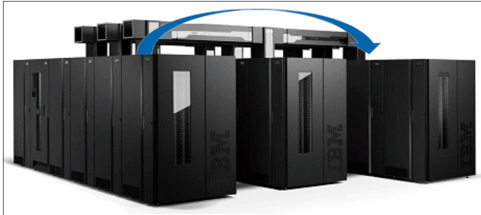
Figure 4-44 TS3500 Shuttle Complex moves tapes cartridges between physical libraries
