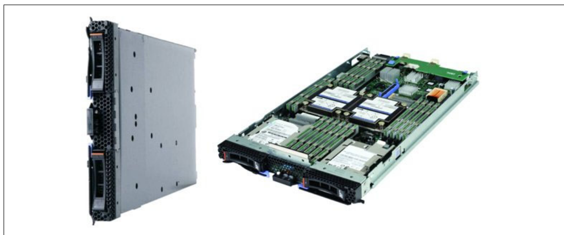
Figure 3-4 View of HS23 BladeCenter module
