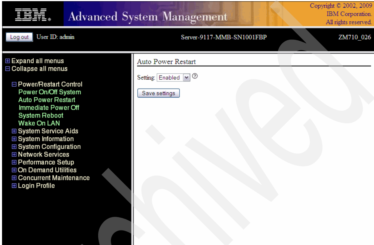
Figure 4-4 ASMI Auto Power Restart setting window interface
