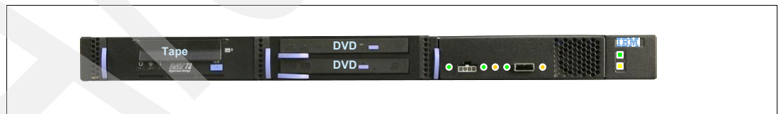
Figure 2-44 DVD/Tape SAS External Storage Unit (#5720)
