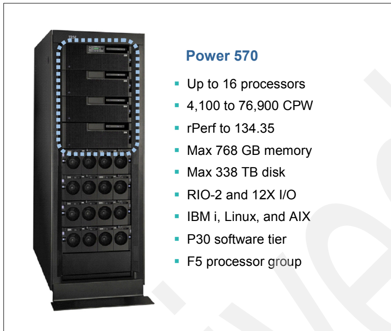
Figure 2-1 9117-MMA 16-Way system rack example
