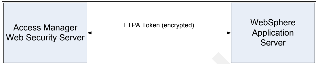
Figure 17 SSO to WebSphere Application Server using LTPASSO to Domino Server
