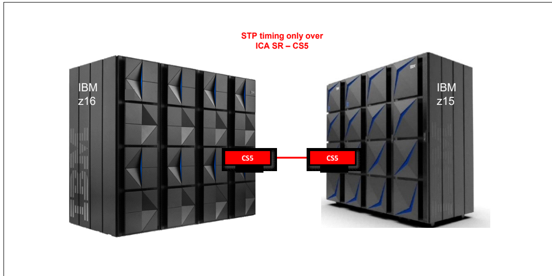
Figure 9-12 STP timing-only link connection from an IBM z16 to an IBM z15 (over CS5)
