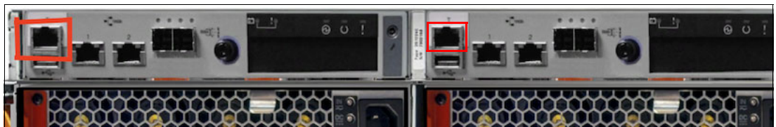
Figure 2-5 Technician port FlashSystem 5045
