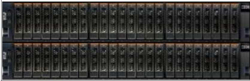
Figure 2-17 HPFE Gen3 enclosure
