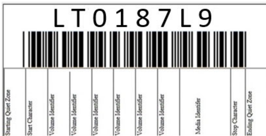
Figure 2-4 Example of an LTO 9 tape cartridge label and its components
