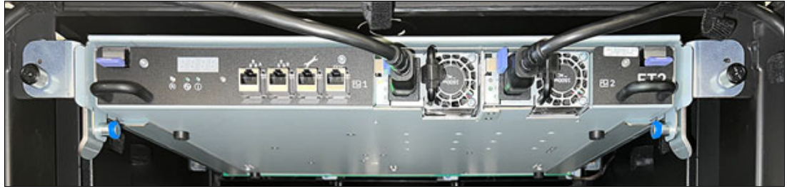
Figure 1-4 IBM Diamondback electronics tray close-up
