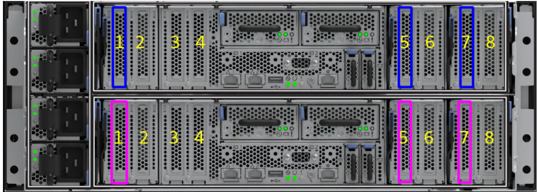
Figure 8-3 Dual Port 100 GbE adapter placement on IBM Storage FlashSystem 9500
