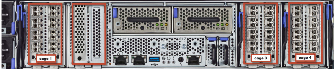
Figure 2-11 SV3 node layout
