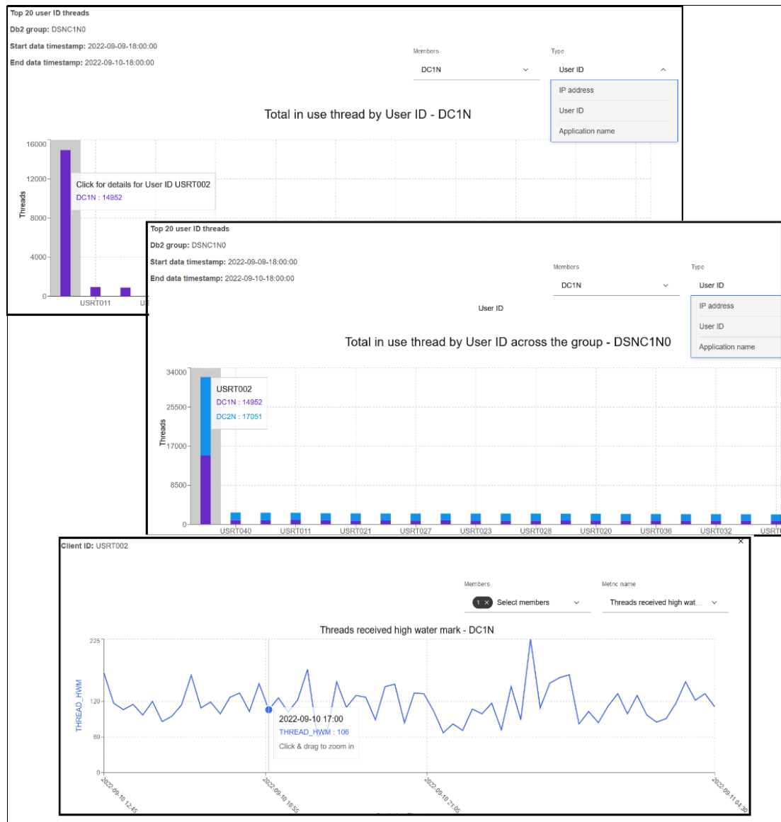
Figure 13-22 DCC dashboard: DBAT high water mark and drilling down to thread statistics
