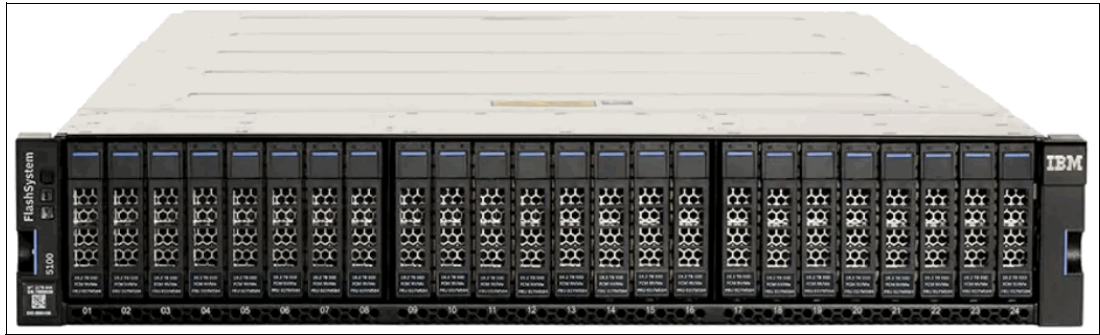
Figure 1-5 IBM Storwize V5100 front view
