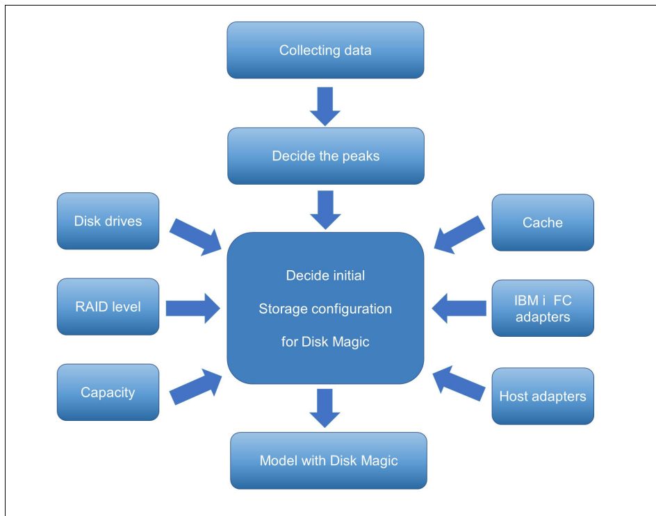
Figure A-9 Diagram of sizing and modeling for IBM i using Disk Magic.
