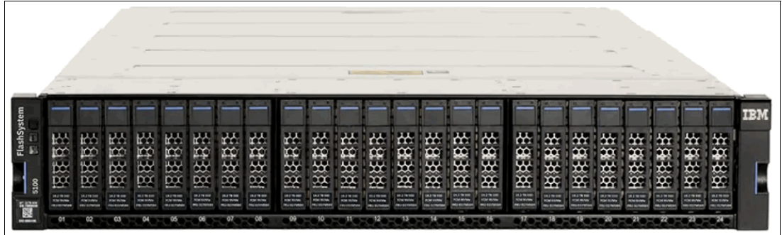
Figure 1-10 IBM FlashSystem 5100 front view showing the 24 NVMe drives installed
