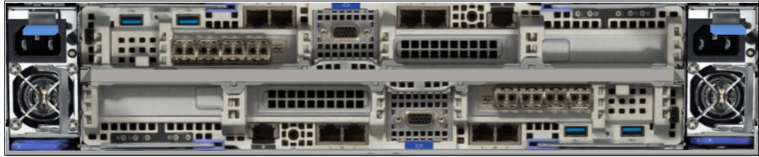
Figure 1-28 Rear view of an IBM FlashSystem 5100 Control Enclosure
