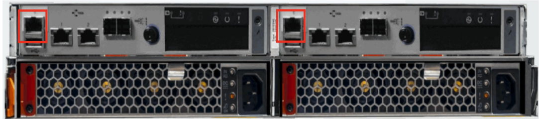
Figure 3-3 Location of the technician port on IBM FlashSystem 5030
