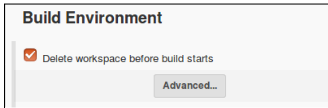
Figure 9-53 Configure the workspace to be removed before building
