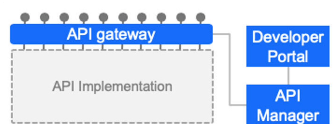
Figure 3-7 API management: More than just a gateway
