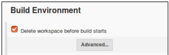
Figure 9-60 Configure the workspace to be removed before building
