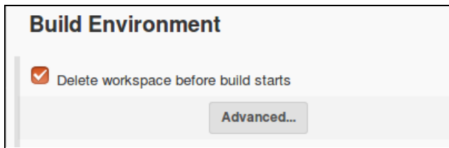
Figure 9-45 Configure the workspace to be removed before building
