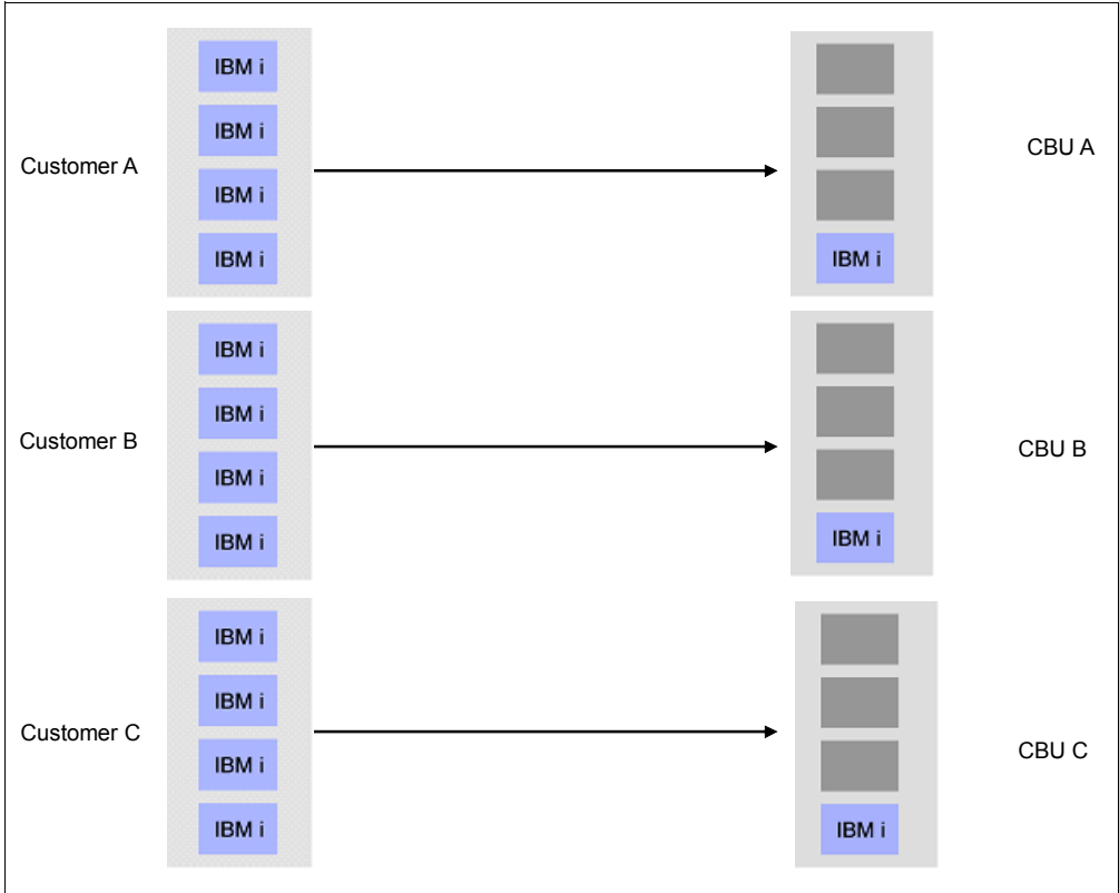
Figure D-5 MSP setup that uses basic CBU topology
