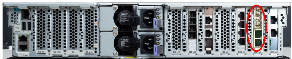
Figure 4-2 Location of the 10 Gbps Ethernet cards in 2U DS8884 servers
