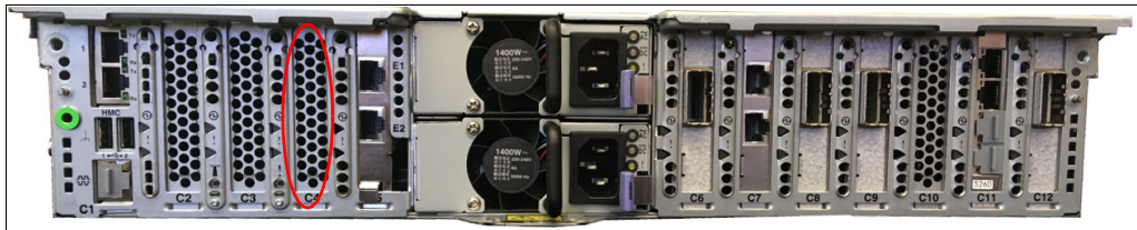
Figure 4-4 Location of 10 Gbps Ethernet card in 2 U servers (DS8910F model 994)
