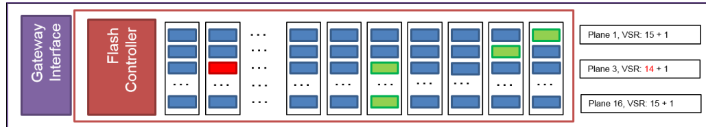
Figure 3-34 FlashSystem Variable Stripe RAID (VSR)
