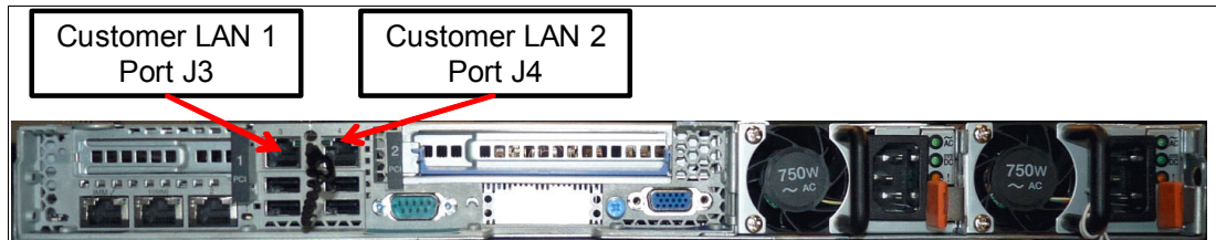
Figure 11-11 SE Physical connection
