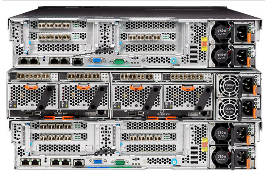
Figure 2-13 IBM FlashSystem V9000 rear view
