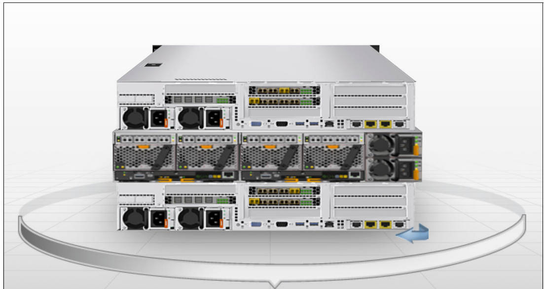
Figure 8-5 Rear view of an AC3 control node based single building block
