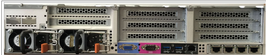
Figure 4-8 AC3 control enclosure rear view.
