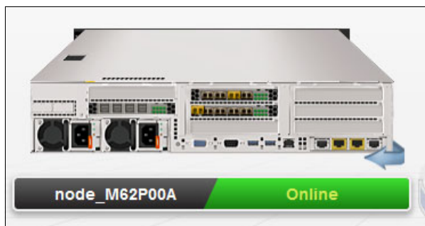
Figure 5-35 AC3 control enclosure rear side
