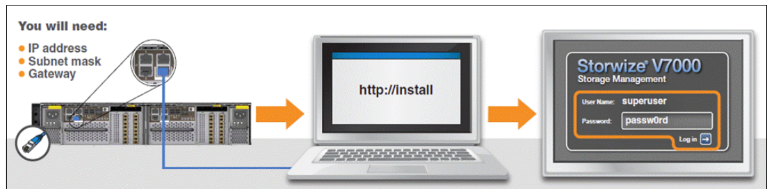
Figure 2-13 Technician port setup
