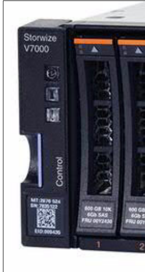
Figure 2-9 Front Control Enclosure LEDs
