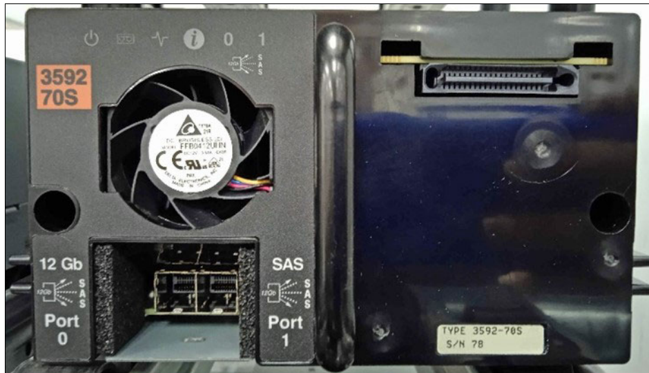
Figure 2-5 TS4500 3592 70S drive rear view
