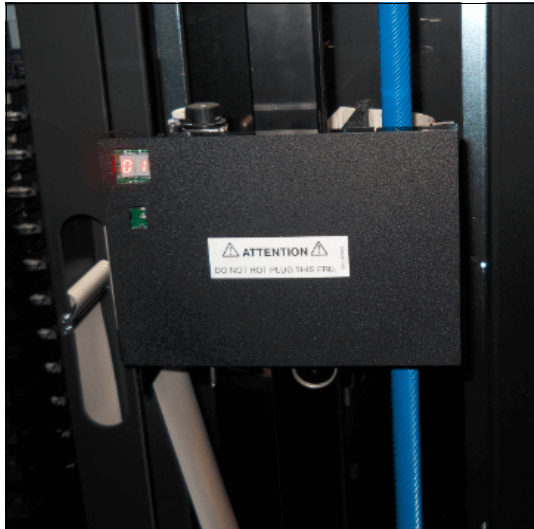
Figure 1-32 Accessor controller (accessor control card)
