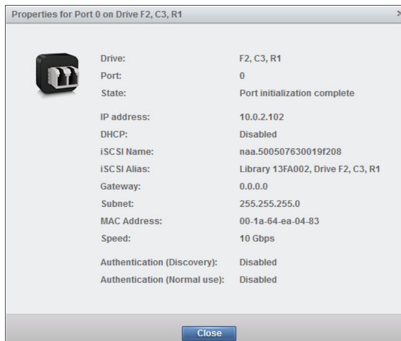
Figure 4-132 Ethernet port properties
