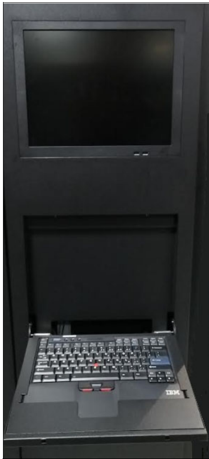
Figure 4-1 The Integrated Management Console
