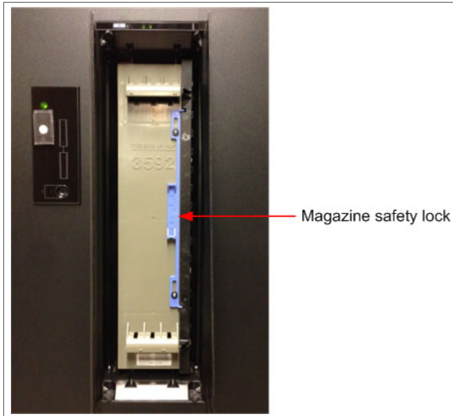
Figure 1-38 Tape cartridge magazine safety lock
