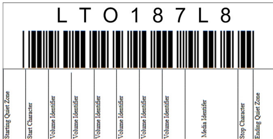
Figure 2-15 View of the LTO-8 tape cartridge label
