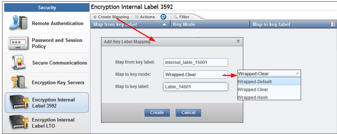
Figure 4-54 Adding or modifying the key label mapping for 3592
