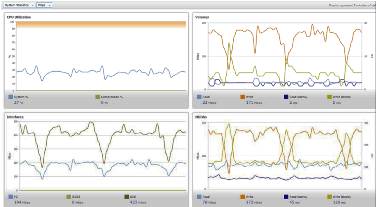
Figure 2-52 IBM Storwise V7000 performance for split mirror non-compressed volumes (MBps)
