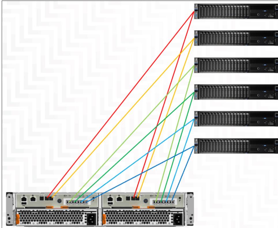
Figure 2-8 Storwize V5020 SAS host attachment
