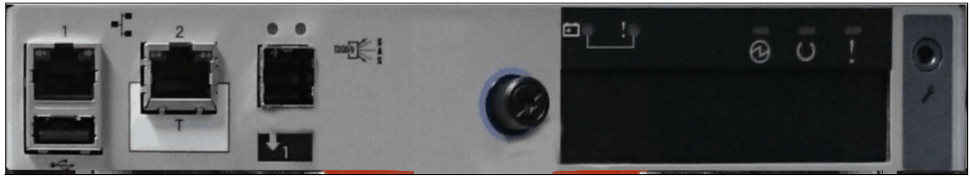
Figure 1-6 Storwize V5010 node canister
