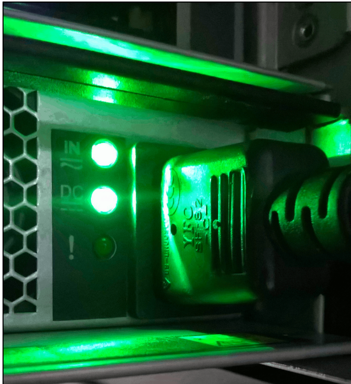
Figure 12-23 PSU status LEDs
