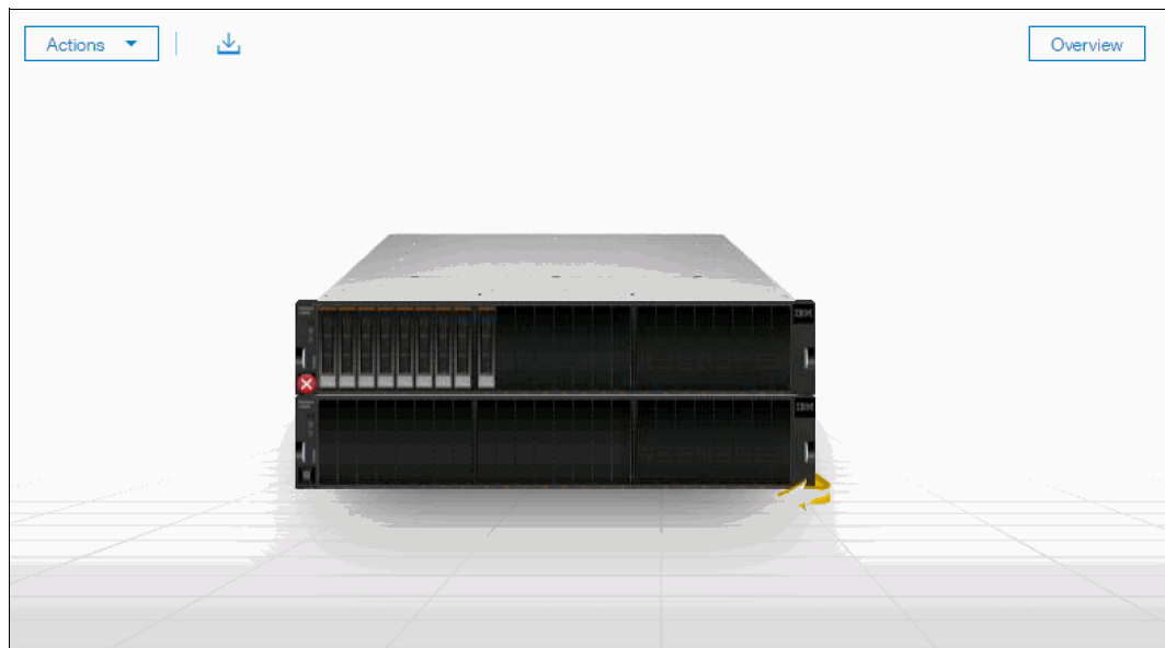
Figure 2-49 IBM Storwize V5000 Gen2 GUI with two enclosures in a single I/O group
