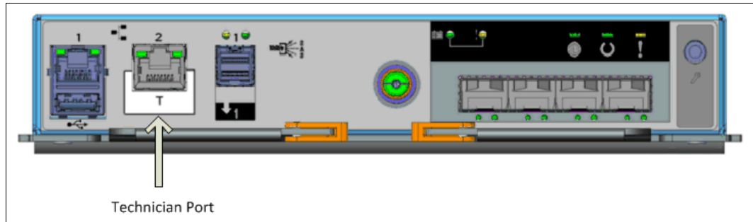
Figure 2-13 Storwize V5010 technician port
