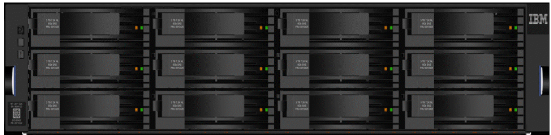
Figure 1-1 IBM Storwize V5000 Gen2 front view for 2077/2078-12 and 12F enclosures
