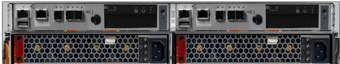
Figure 1-4 Storwize V5020 control enclosure rear view
