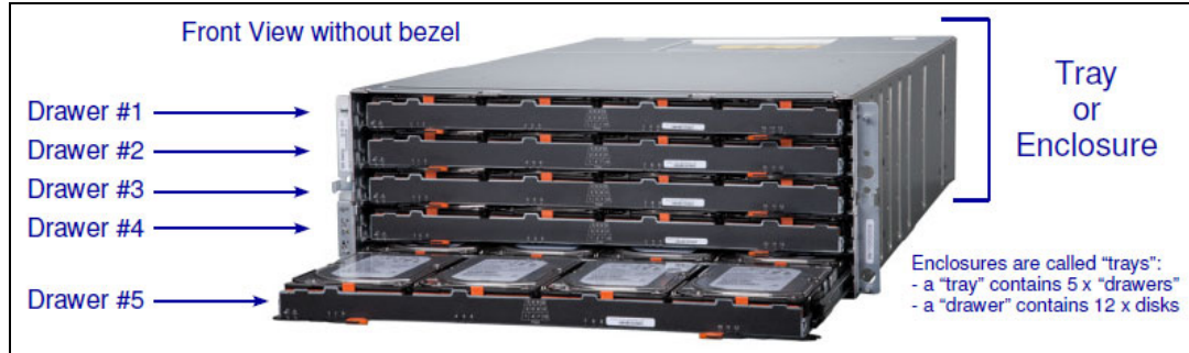
Figure 4-34 IBM DCS3700 4U chassis and drive trays
