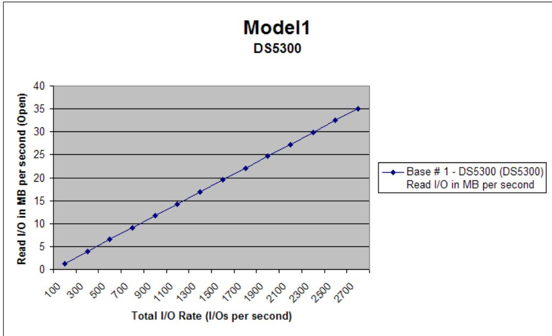
Figure 10-41 Output from read I/O versus I/O rate graph
