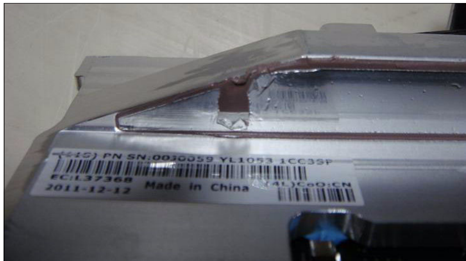
Figure 4-11 Compute card TIM with damaged foil
