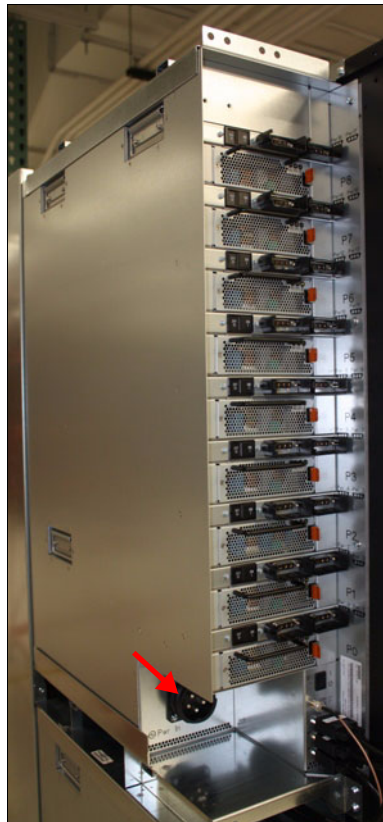
Figure 1-13 Power lead connector on a BPE
