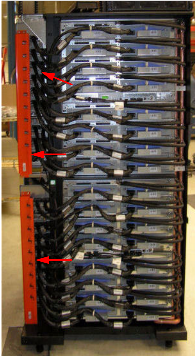
Figure 1-1 Blue Gene/Q shipping bracket placement
