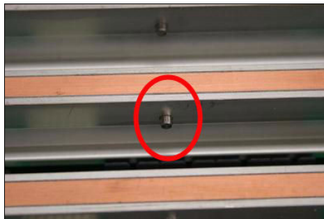
Figure 4-15 Latch pin for a compute card on a node board
