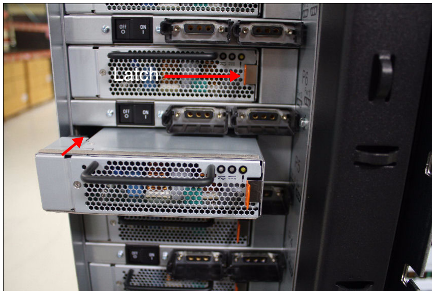
Figure 1-18 BPM installations and latch
