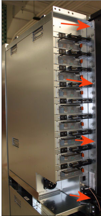
Figure 4-31 BPE retaining screw locations
