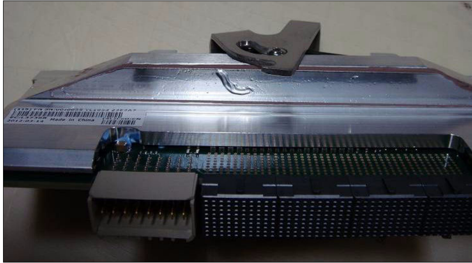
Figure 4-12 Compute card TIM with large indentation
