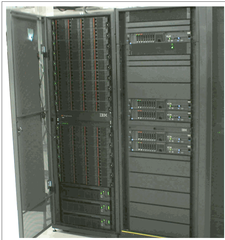
Figure 3-4 Small configuration of a SONAS Gateway with one XIV
