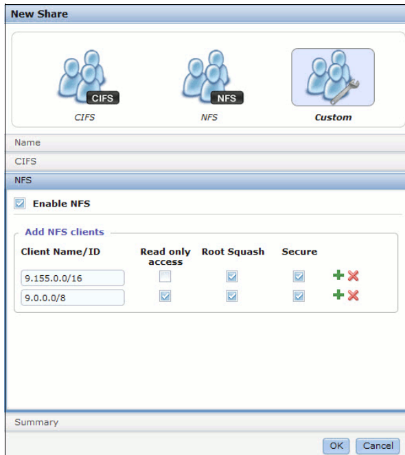
Figure 2-34 The NFS window allows setting the NFS client names or IP ranges
