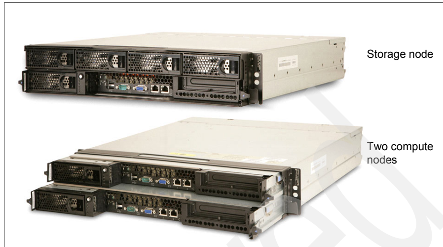
Figure 2-48 Two possible configurations of the iDataPlex 2U Flex chassis
