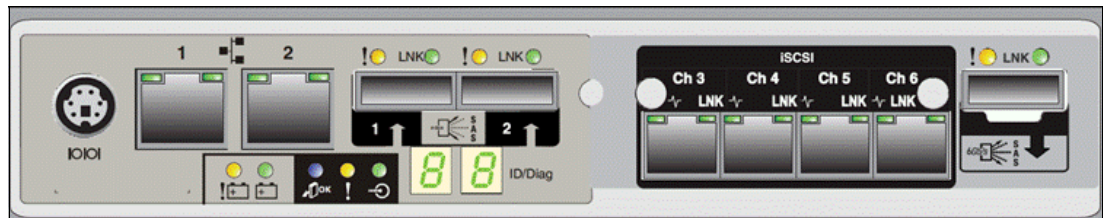
Figure 4-4 The rear panel of a DS3500 controller with the optional iSCSI host port adapter installed
