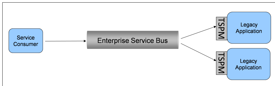
Figure 5-2 Established application solution
