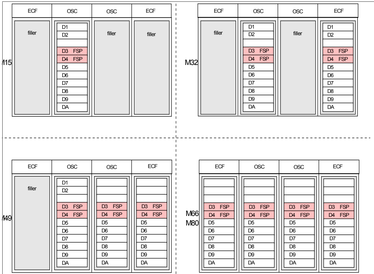
Figure 4-12 Fanout plugging rules
