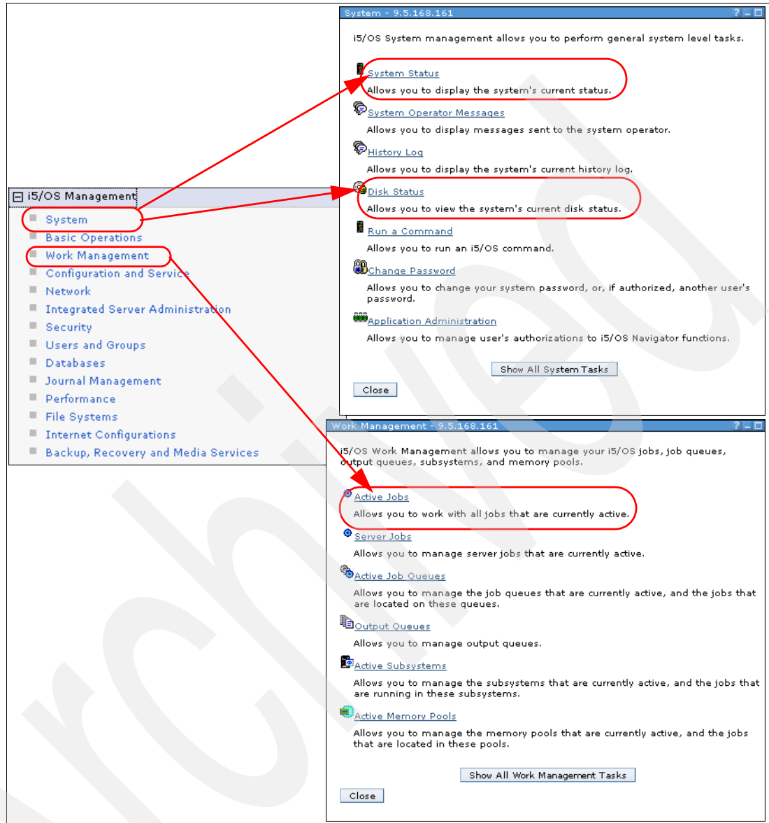
Figure 6-19 Alternate path to get to real-time performance
