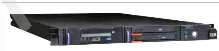
Figure 11-18 7214 Storage Device Enclosure
