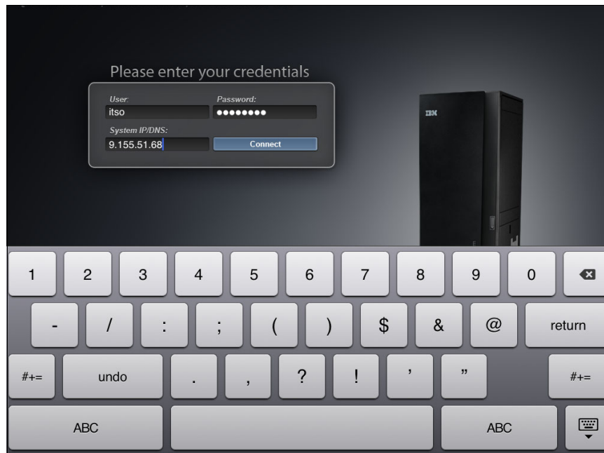
Figure 7-30 Logging on to an XIV Storage System from the IBM XIV Mobile Dashboard
