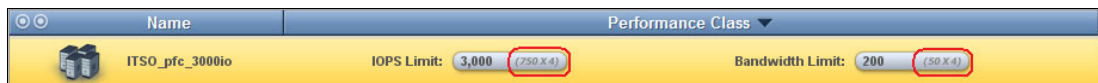
Figure 4-70 QoS, calculation based on active XIV interface modules (9-module XIV Storage System)
