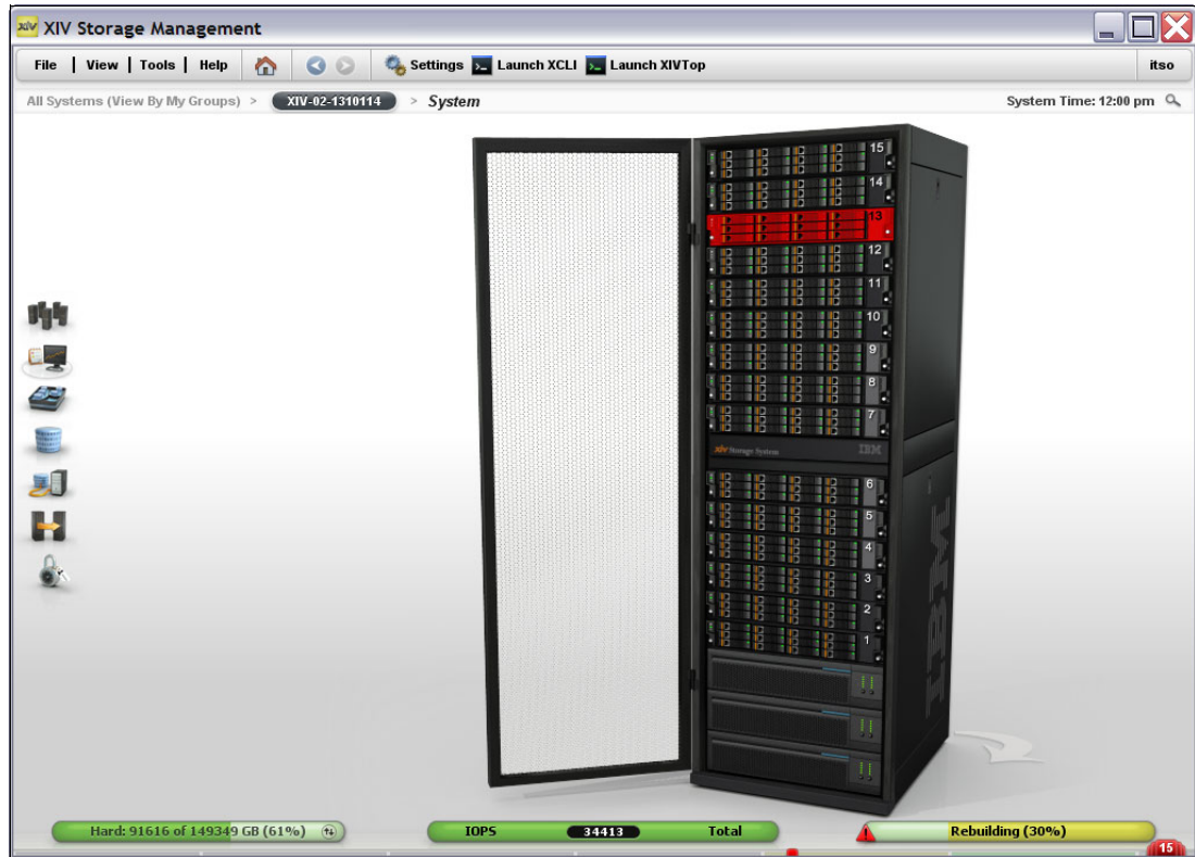
Figure 2-12 Rebuilding status in the XIV Storage System GUI
