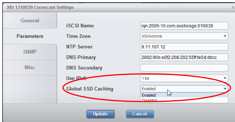
Figure 4-118 System settings for Global SSD Caching
