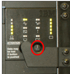
Figure 3-34 Locate Test button
