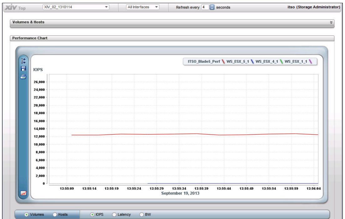
Figure 6-25 Display performance information for up to four volumes or hosts with XIV Top
