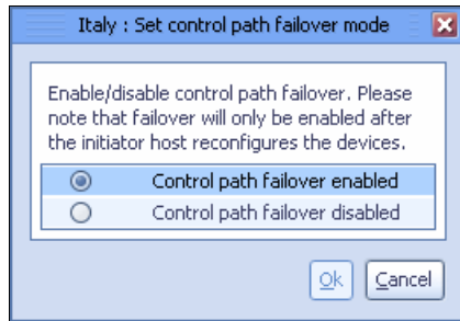
Figure 6-20 Set control path failover mode
