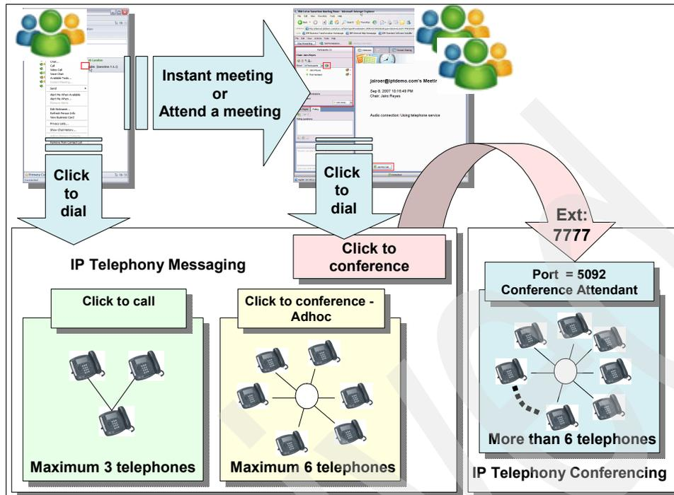
Figure 3-2 IP Telephony Collaboration functions with Sametime
