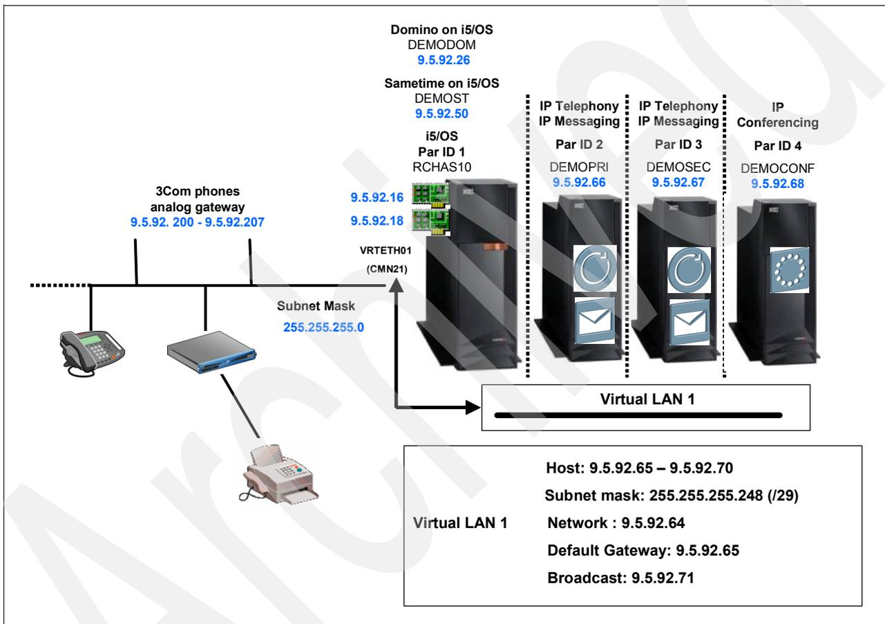
Figure 1-13 The System i test environment used in this book
