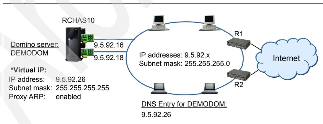
Figure 1-1 Domino server configured with a virtual IP interface
