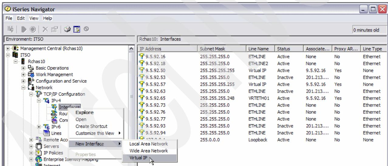
Figure 1-2 Starting the New IPv4 Interface wizard
