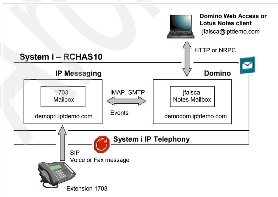
Figure 4-1 Unified inbox solution with Domino and System i IP Telephony
