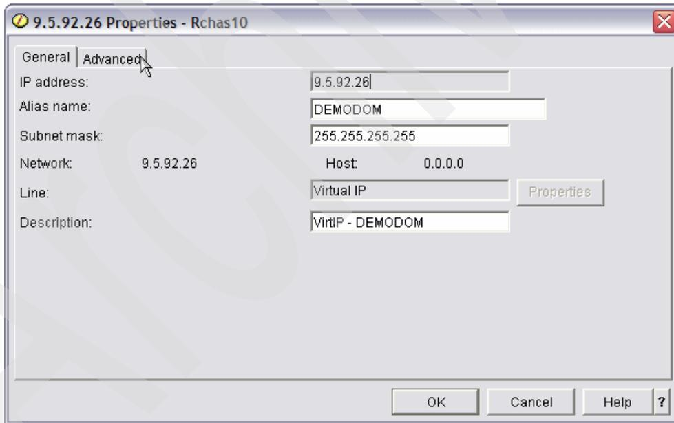
Figure 1-8 Virtual IP interface properties
