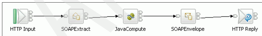
Figure 6-29 Use SOAP nodes to make the message flow a Web service provider
